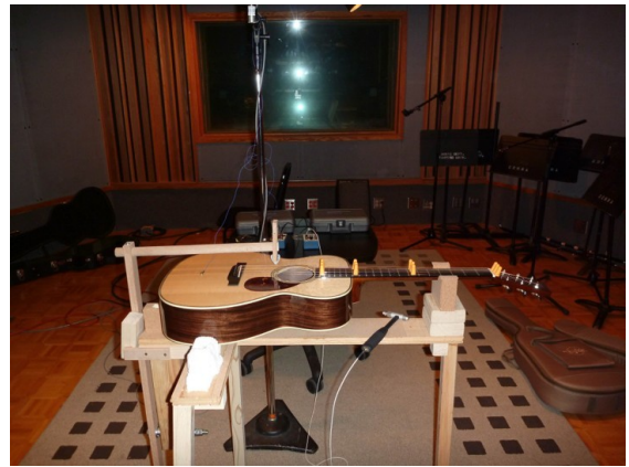
Photo 1 - Guitar testing set-up, showing instrumented hammer, accelerometer mounted to guitar top, microphone, guitar cradle, strumming apparatus and foam string dampers.
