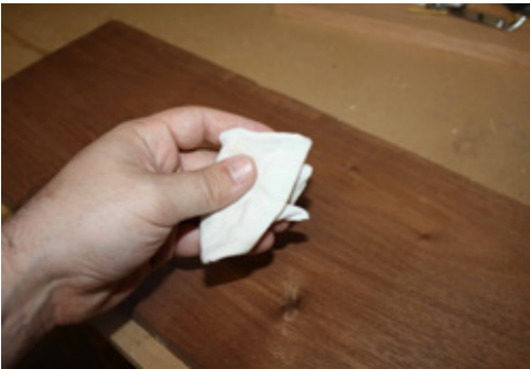
Any white cotton cloth can be used with Naphtha to remove steel wool residue.
