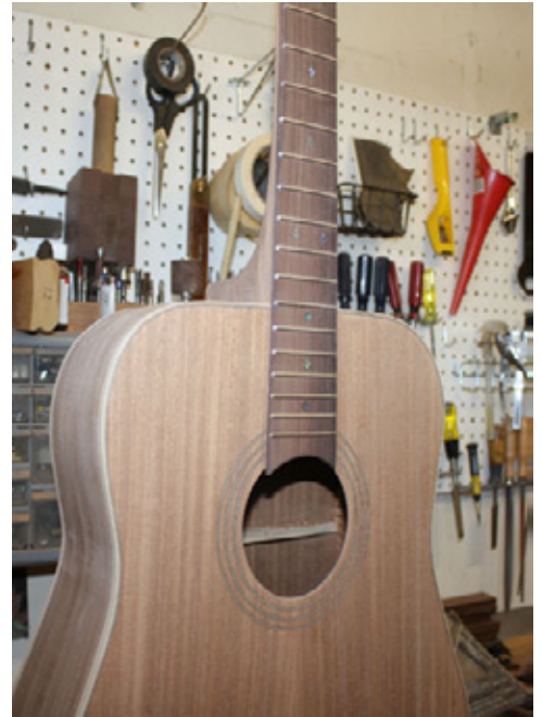
This guitar is completely unfinished, and the term “in the white” is used to refer to completed instruments that are awaiting a finish.
