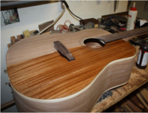
This guitar has one half of the top coated in an oil finish. Notice how the coloring really comes out after the oil is applied.
