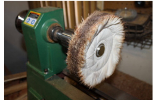
This is a lathe mounted buffing wheel that is held in place with a chuck.
