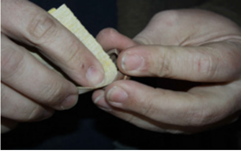
Sanding a ring with 220 grit to smooth out the area where the 120 grit was used, and finalize the surface.
