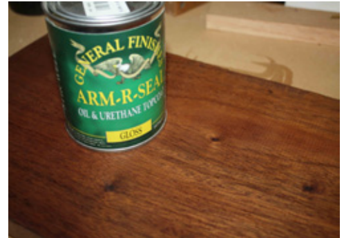
Arm-R-Seal finished board after 0000 steel wool.
