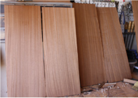
Mahogany is an example of an open grain wood, because the pores are easily visible on the surface.
