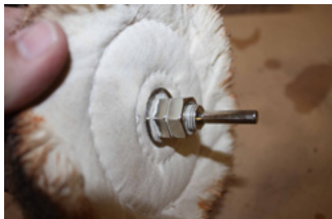
This is a store bought buffing wheel with a basic mandrel that can be held in any chuck.
