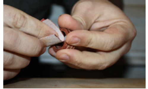
Sanding a wooden ring with 120 grit paper to quickly break a sharp edge on the inside of the piece.
